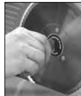
Figure 7. Turn the screw clockwise for blade removal.
