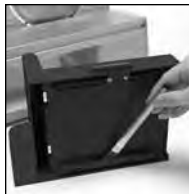
Figure 6. Lubricating food carriage guides.
