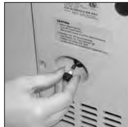
Figure 10. Replacing the fuse located underneath motor housing.
