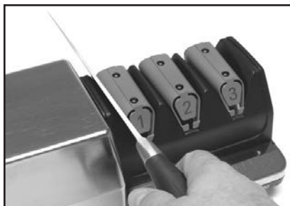
Figure 5. Stage 1. Inserting blade in slot between guide and knife hold down spring. Alternate left and right slots.
